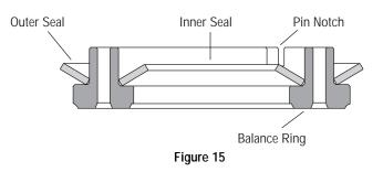
**38** Align pin notches in balance ring with pins in bore of valve housing. Install balance ring assembly in valve housing.
