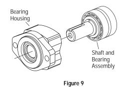
**19** You may need a press to remove shaft and bearing assembly from bearing housing. (Key must be removed before removing shaft.)
