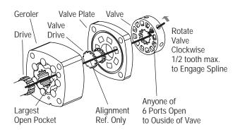
Figure 12 Timing Alignment
