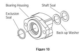
**20** Use a small screwdriver to remove shaft seal, back-up washer and exclusion seal from bearing housing, see Figure 10. Do not damage bore of housing.
